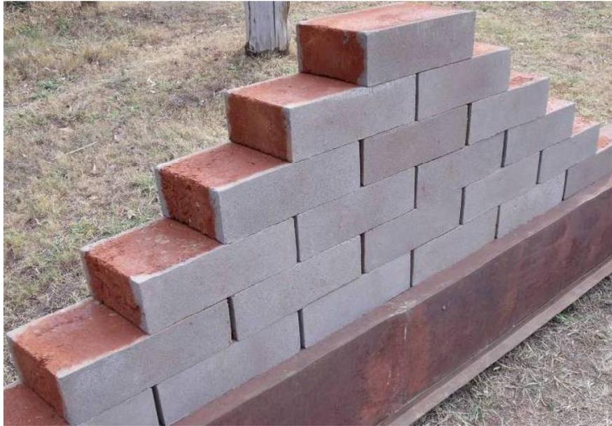
A SCCB consumes less cement than a usual stabilized earth block. However, a building made with SCCB has the same appearance than the one constructed with cement blocks, even better.
